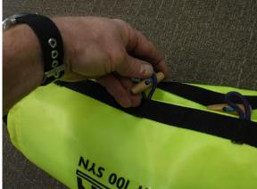
The inner baffle is brought over the packed rope and secured with the attached Velcro. The outer flap is then closed and secured with the toggles. Note: the toggles allow secure fastening in severe weather conditions (mud, snow, low temps) where zips or Velcro may not be effective
